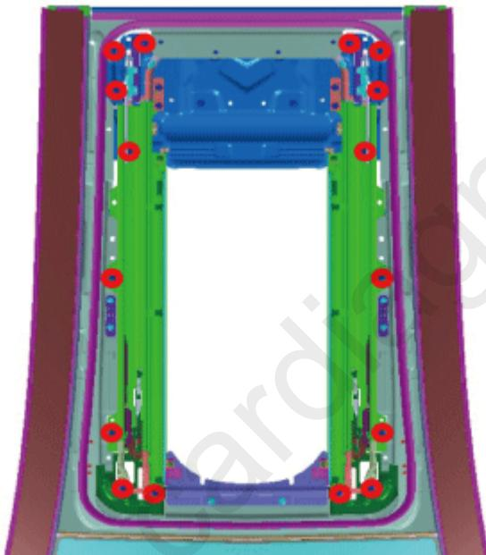
11. Remove the mechanism rail assembly(A).
