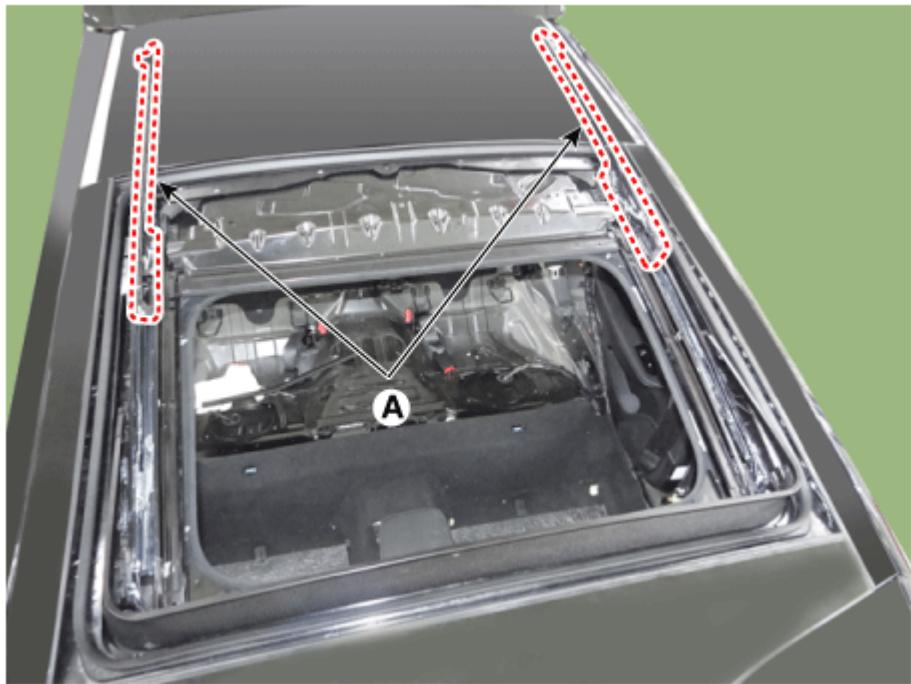
3. Open the glass motor as maximum by pressing sunroof switch after IG is ON.
