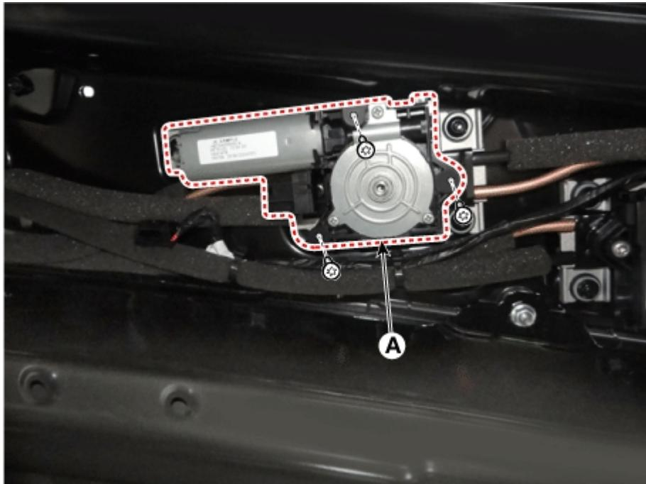
10. Loosen the mechanism assembly mounting screws.
