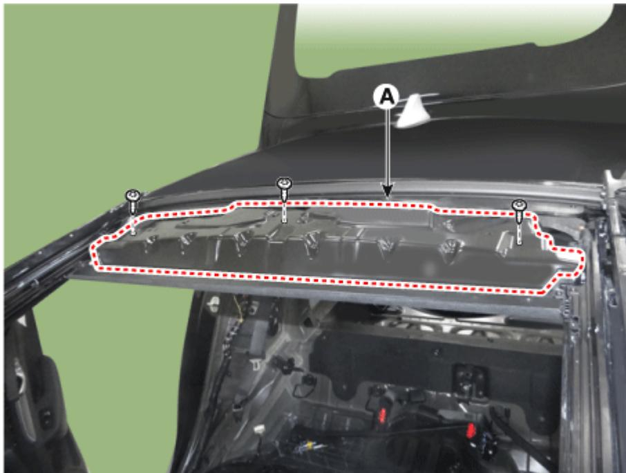
8. Disconnect the roller blind motor and the moving glass motor connector.
