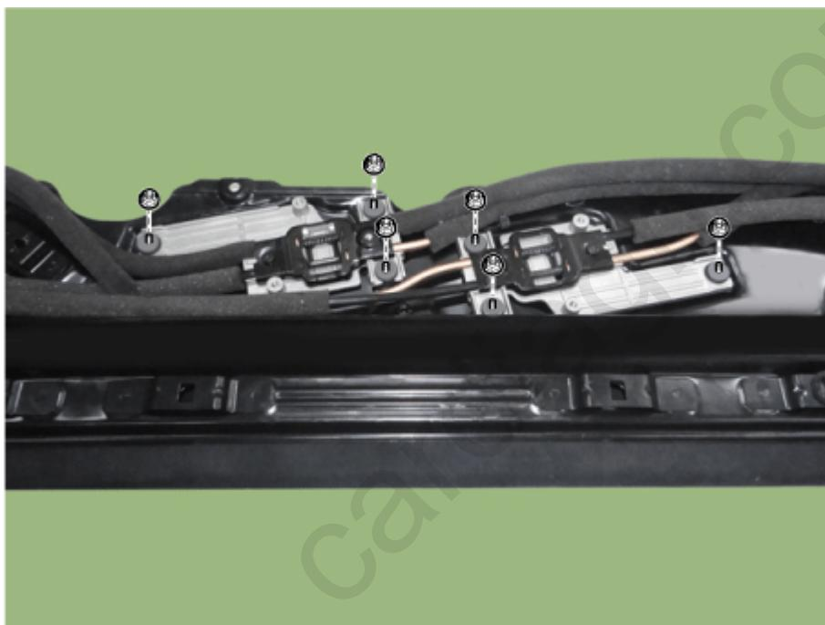
18. Loosen the roller blind mounting screws.
