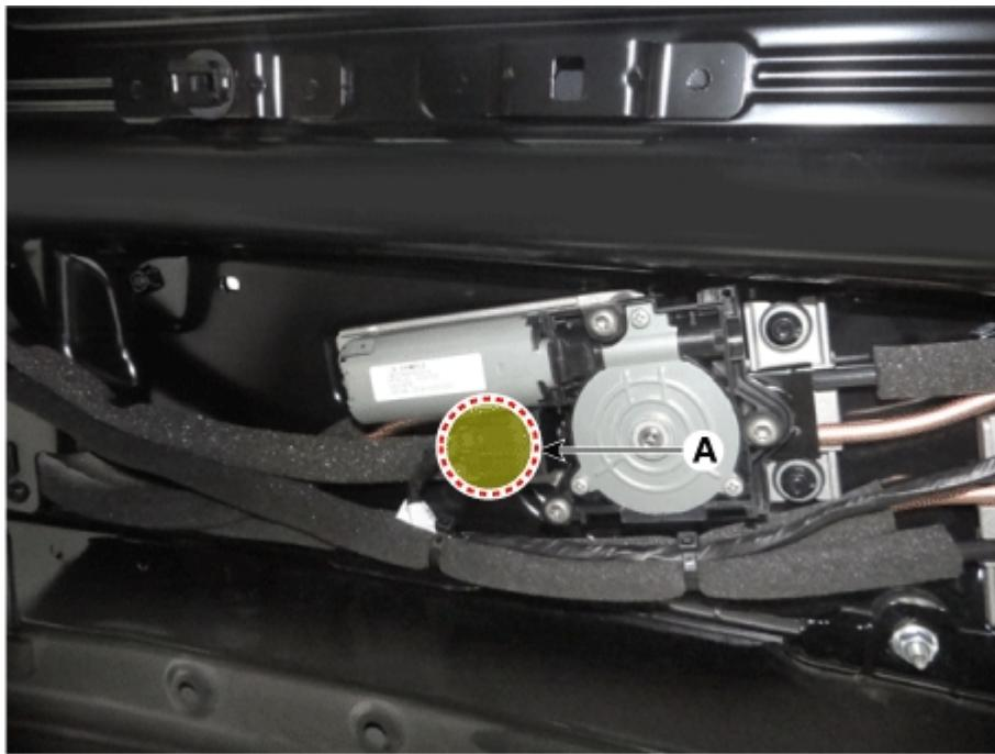
9. Remove the roller blind motor and the moving glass motor after loosening the mounting screws.
