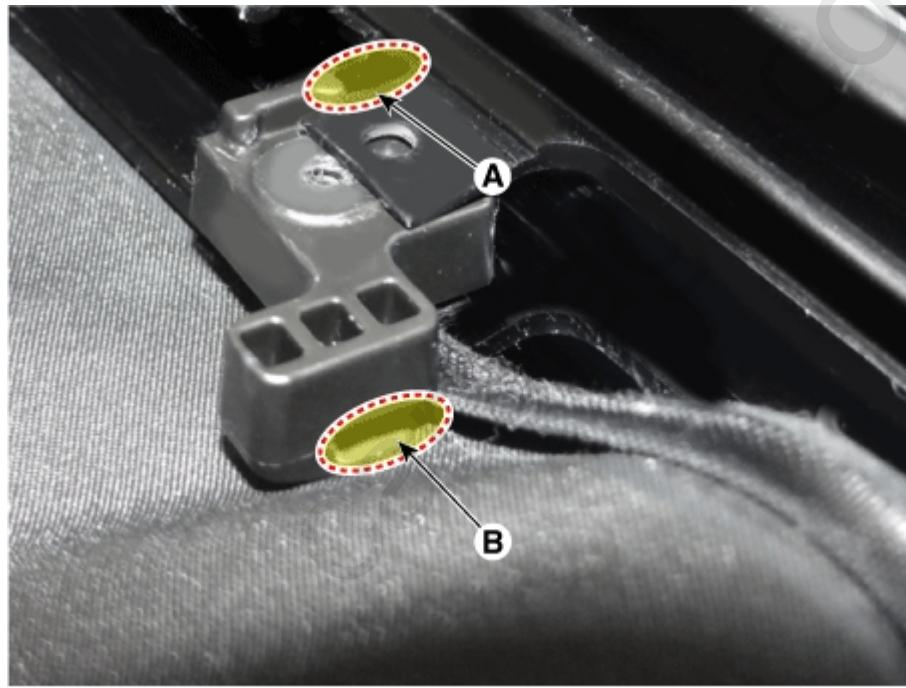
14. Loosen the roller blind shoe clip mounting screw (A).
