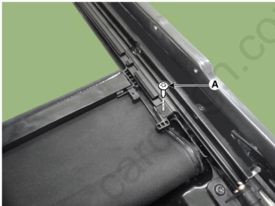
13. Remove the roller blind lead (A) from the mechanism rail.
