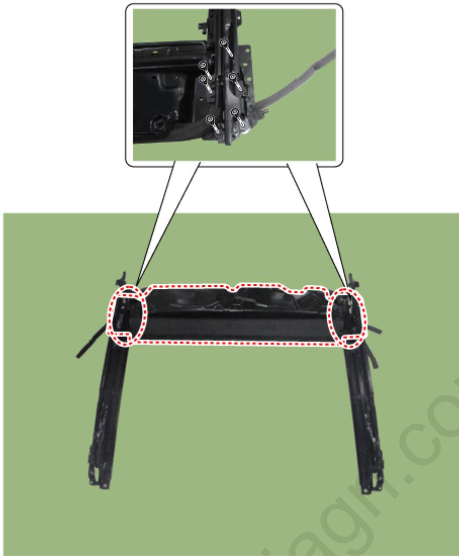
19. Remove the roller blind(A) from the mechanism rail.
