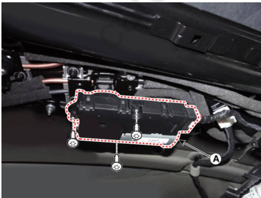
2. Open both mechanism assembly (A) as much as possible.
