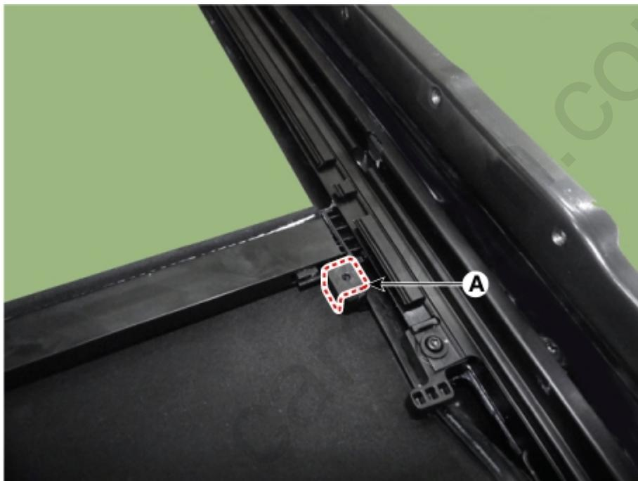
16. Remove roller blind bar (B) by pressing locking pin (A) with using flat-tip screwdriver.
