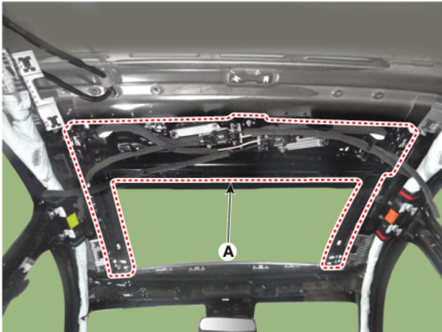
12. Loosen the roller blind lead mounting screw (A).
