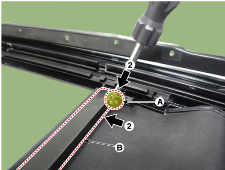
17. Loosen the drive unit mounting nuts.
